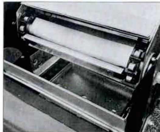
**Grain Saver.** A simple, yet effective device that works in conjunction with tilt-up hopper to prevent grain spillage.
