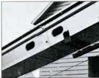
**Anti-Sag Construction.** Sturdy, rust-resistant galvanized steel trough sections are connected with embossed, interlocking joints. All section joints are reinforced to prevent sagging. Cadmium-plated bolts and nuts add extra corrosion resistance.
