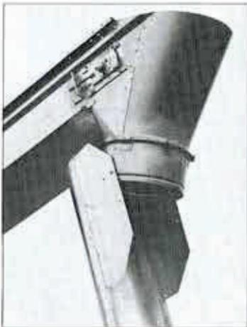
**360° Swivel Head and Telescoping Spout** fills crib corners. Aim the flow where you want it. Large 18" diameter opening. Telescoping 4' downspout sections increase reach up to 16'. Assembly can be swung out of the way, or removed, for bale handling.
