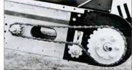
**Adjustable Speed Reduction** with optional Opposite Side Drive lets you drive the elevator from either side. Slip clutch can be adjusted for elevating various materials.
