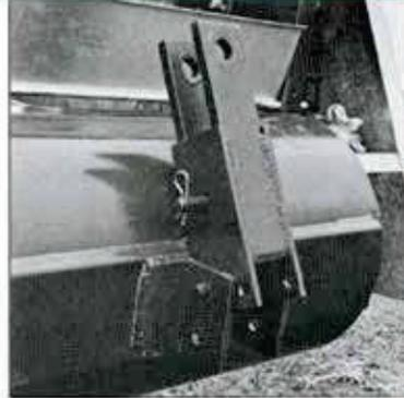
**Double Clevis Hitch.** Strong and rigid for towing. Change pin and swing out of the way when working.
