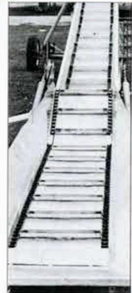
**Full Width Trough** opening, at 20 1/2" wide and 7" deep. Allows bales to move freely from hopper to elevator.
