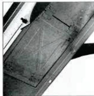
**Corn Screen/Relief Door.** Standard features. Located in top section of elevator for maximum cleaning. Open the relief door to allow discharge of screened material. Leave closed while elevating small grains.
